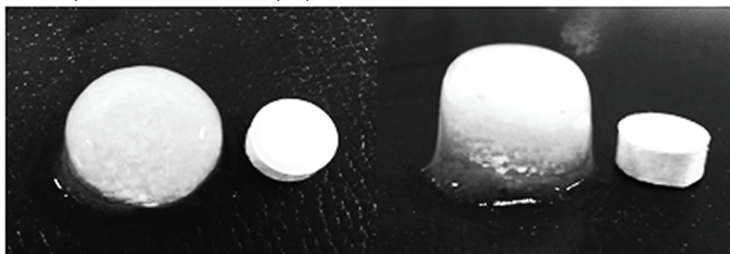
Figure 8 The shape of famotidine matrix tablets after in vitro dissolution test.
