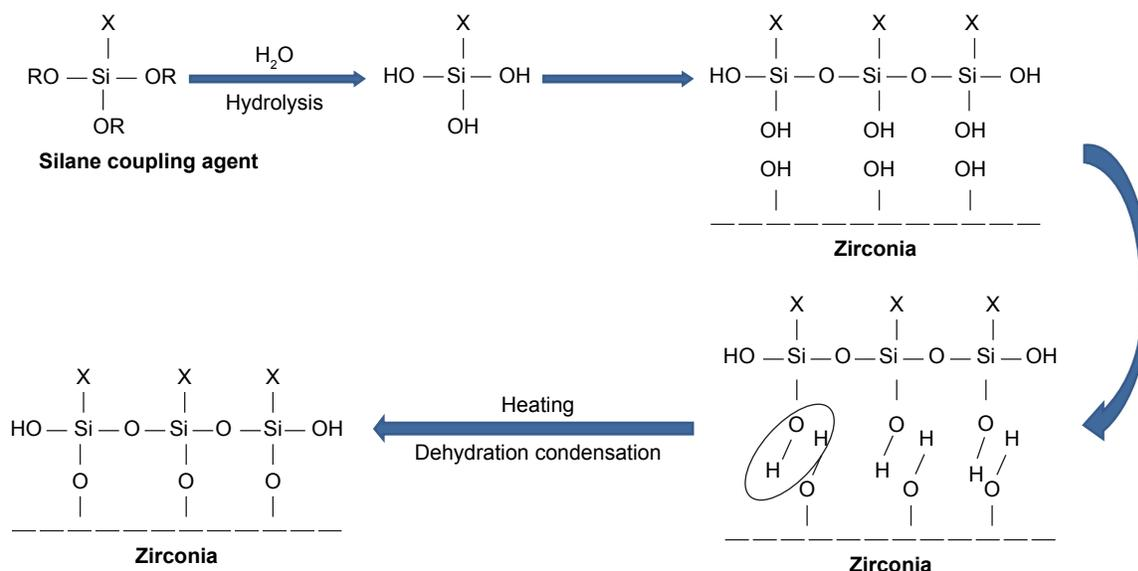
**Figure 2** Schematic diagram of silanization of nano- $\text{ZrO}_2$ .
