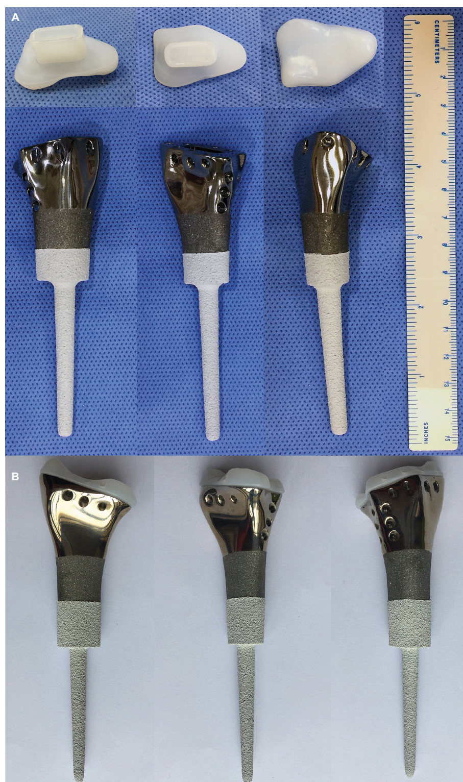
Figure 4 (A) Components of prosthesis; (B) endoprosthesis with HA coating. Abbreviation: HA, hydroxyapatite.
