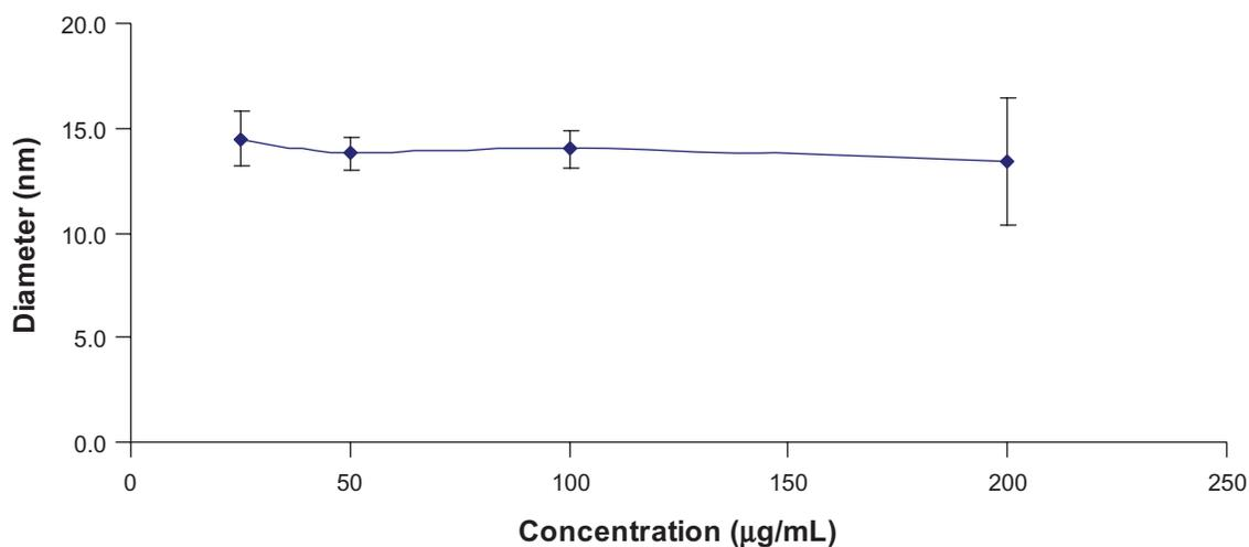
**Figure 3** Critical micellar concentration of PGG-PTX nanoconjugate. The DLS could not detect the particle size of PGG-PTX solution below 25 µg/mL. The critical micellar concentration was assumed to be about 25 µg/mL in saline at 25°C. The results are expressed as means  $\pm$  SD ( $n = 3$ ).
