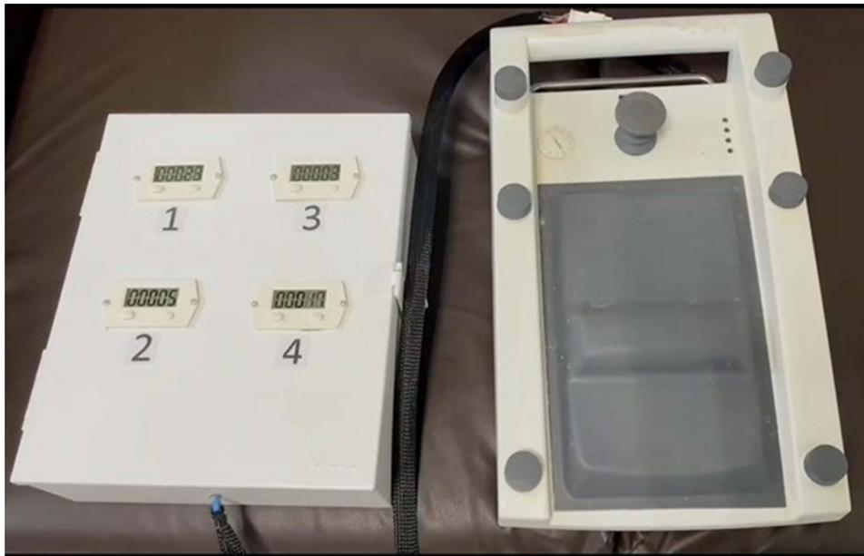
**Figure 1** Counter connected to the microscope footswitch.
