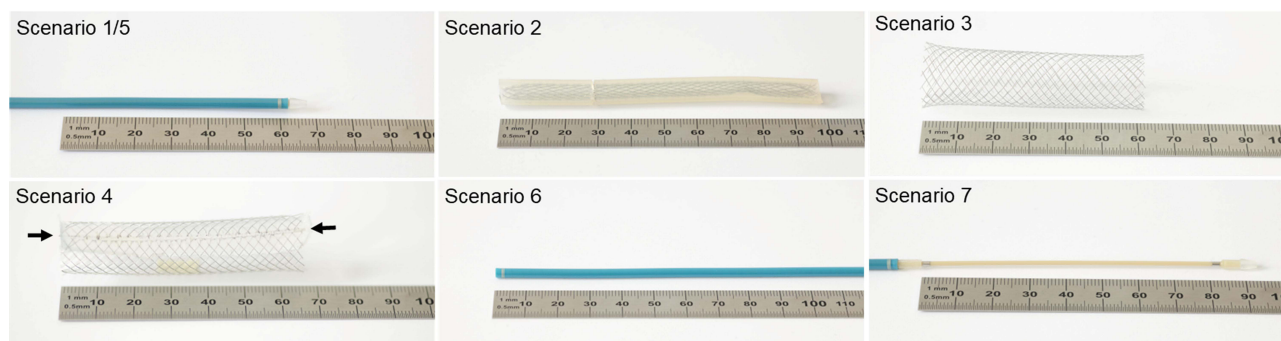
Figure 1 Images of the seven different measurement scenarios of the stent and its delivery system. Scenarios 1 and 5 are represented by the same photography since the delivery system looks identical from the outside before and after stent implantation as the stent is covered by the blue part of the delivery system before deployment.
