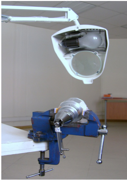
Figure 3 The torque gauge was fixed in a vice for stability and aligned with a magnifier.
