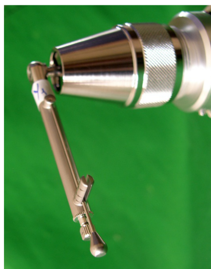
Figure 2 Drivers for each of the S-S MTDs were clamped in a three-jaw chuck of a torque gauge.
