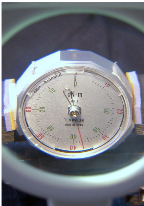
Figure 5 Peak torque values of each of the S-S MTDs presented on a torque indicator of the gauge. For each device, peak torque was registered using magnifier. Abbreviation: S-S MTDs, spring-style mechanical torque devices.
