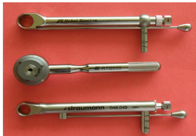
Figure 1 Spring-style mechanical torque devices tested.
