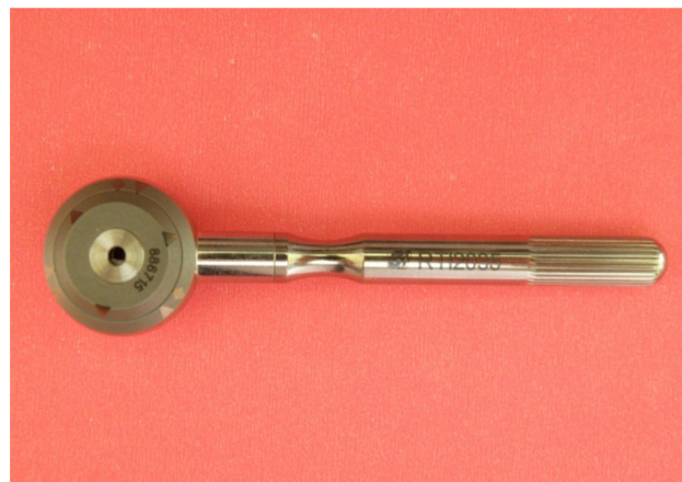
Figure 8 Biomet 3i (Palm Beach Gardens, FL) mechanical torque device.
