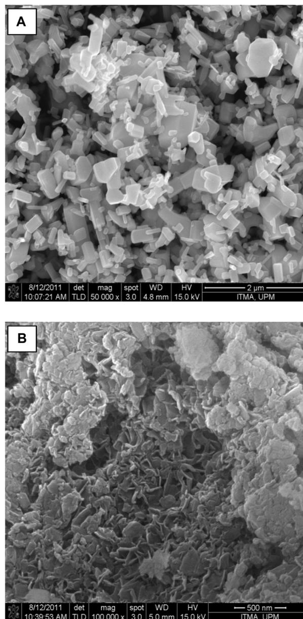
**Figure 6** Field emission scanning electron microscopic images of (A) zinc oxide with 50,000 × magnification and (B) salicylate-zinc layered hydroxide nano hybrid 0.8 mol/L with 100,000 × magnification.
