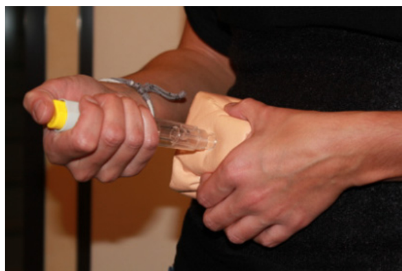
Figure 1 Simulated subcutaneous injections were performed in a foam pad, mimicking skin behavior.
