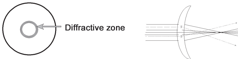
Figure 5 Diffractive SCL. There is a refractive part at the center, which is surrounded by many circular diffractive zones. A distant image is formed by refraction at the center, while a near image is formed in the diffractive zone on the inner surface of the lens.
