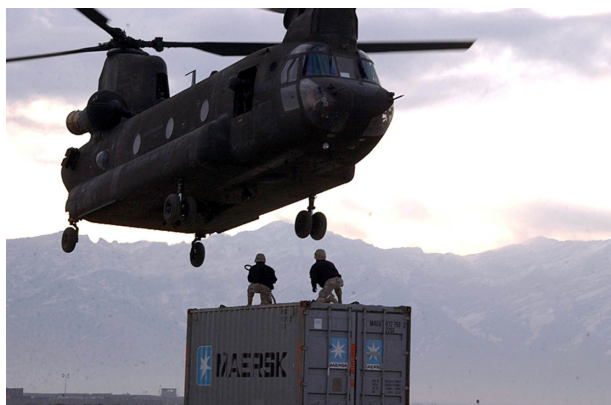
Figure 1 Chinook helicopter used by the US Army and other organizations for transport of cargo containers that can serve as portable operating rooms and other facilities necessary for a disaster response hospital. This helicopter has a payload of 12,000 kg and a range of 1,100 km.
