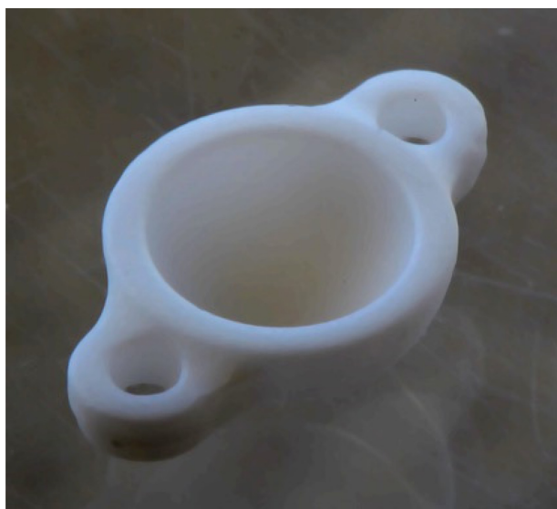
Figure 1 The zirconia space-maintaining device.
