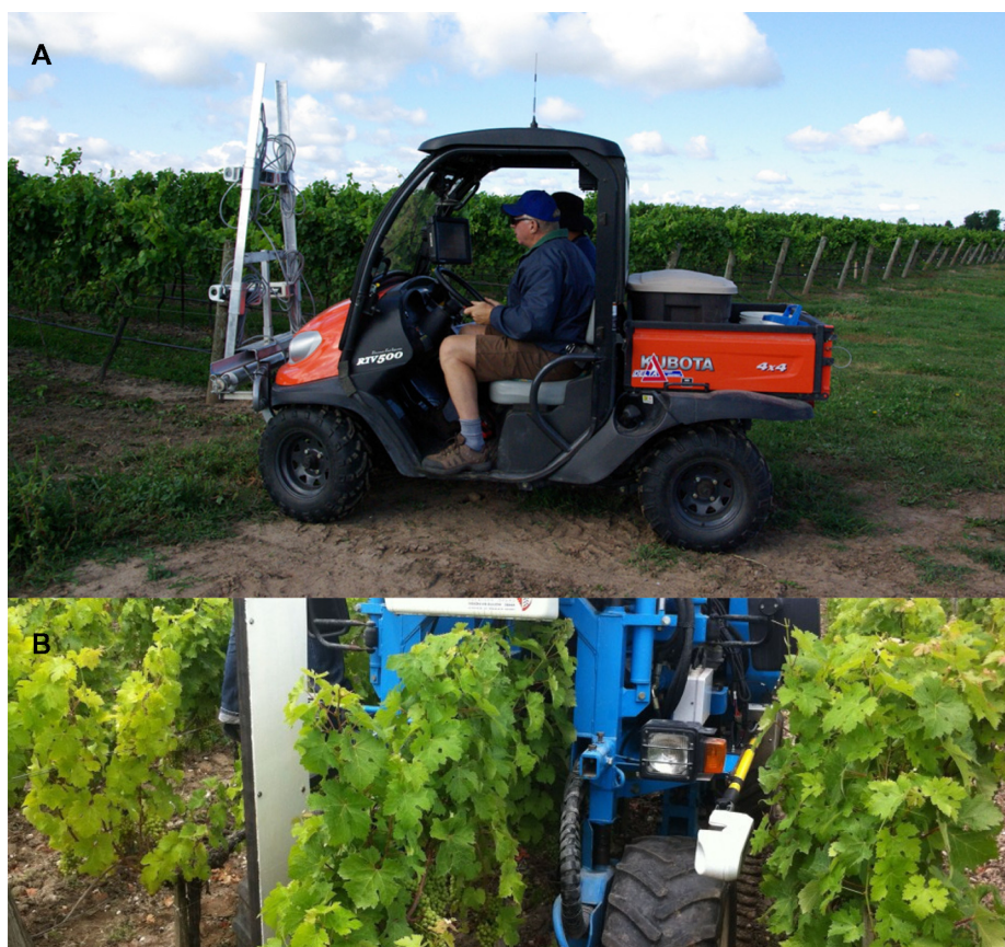
Figure 5 The Trimble® GreenSeeker® multispectral sensor for canopy monitoring, carried on a quad (Practical Precision Inc., Tavistock, Canada) (A) or tractor (Avidorhightech SA, Le Mont-Pèlerin, Switzerland) (B).
