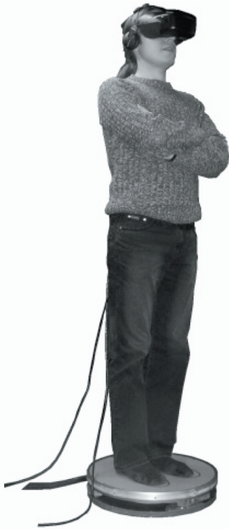
Figure 3 A subject stands on the force platform wearing the stereo display in the virtual reality helmet.
