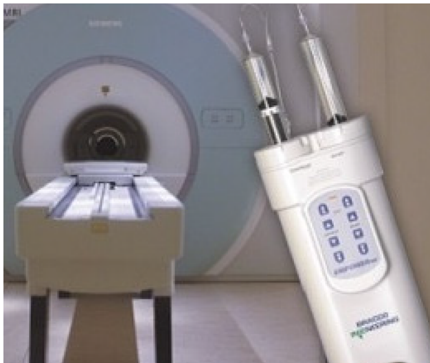
Figure 5 Magnetic Resonance CMI operating at magnetic field strength of up to 9.4 T due to a hydraulic drive.
