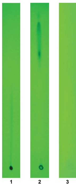
Figure 2 Evaluation of dexamethasone-(C 21 -phosphoramidate)-[anti-EGFR] by analytical HP-TLC for the detection of residual dexamethasone not covalently bound to anti-EGFR immunoglobulin.
