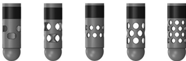
Figure 3 Hole patterns tested for spray capabilities.
