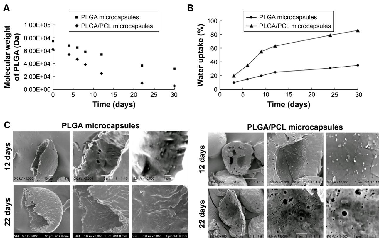
**Figure 4** (A) Average molecular weight of PLGA, (B) water uptake, and (C) SEM images of the degrading PLGA microcapsules and PLGA/PCL microcapsules over time. **Abbreviations:** PCL, polycaprolactone; PLGA, poly(D,L-lactide-co-glycolide); SEM, scanning electron microscopy.
