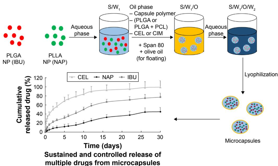
**Scheme 1** Schematic illustration of the encapsulation of NSAIDs into controlled-release microcapsules and the corresponding release of these drugs from the two drug delivery systems (PLGA shell vs PLGA/PCL shell).
