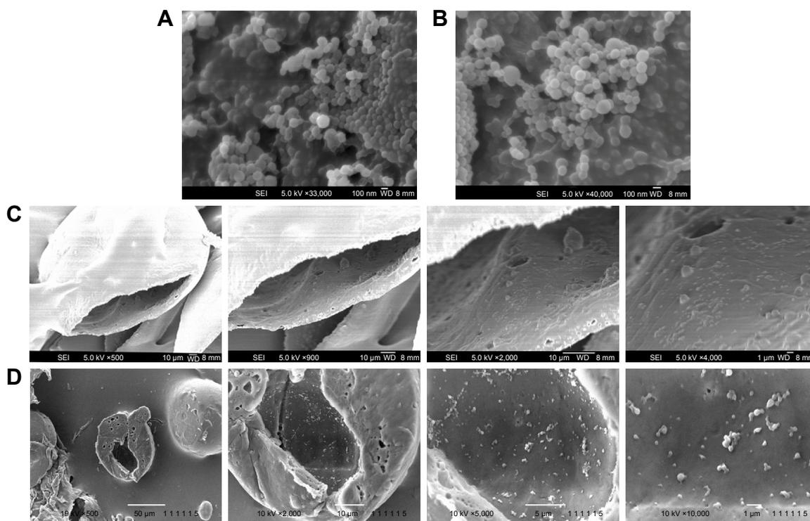
**Figure 2** FESEM images of (A) IBU-loaded PLGA nanoparticles, (B) NAP-loaded PLLA nanoparticles, (C) cross-sectioned CEL-loaded PLGA microcapsules containing PLGA and PLLA nanoparticles, and (D) CEL-loaded PLGA/PCL microcapsule containing PLGA and PLLA nanoparticles. Subsequent magnifications show PLGA and PLLA nanoparticles within the hollow cavity of the microcapsule.
