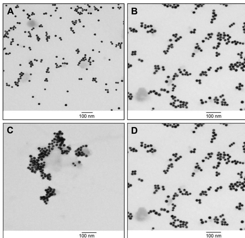
**Figure 3** TEM images of AuNPs: (A) pure AuNPs in citrate buffer, (B) PEP-AuNPs immediately after the synthesis, (C) PEP-AuNPs before centrifugation, (D) and PEP-AuNPs after centrifugation.
