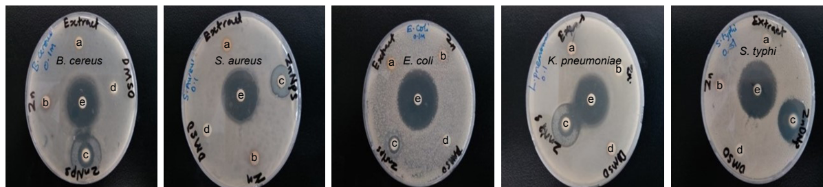
Figure 7 Zone of inhibition of 0.1M synthesized ZnO NPs compared with extract, zinc nitrate solution, DMSO, and antibiotics: (a) extract, (b) zinc nitrate solution, (c) ZnO NPs, (d) DMSO, and (e) antibiotic (ciprofloxacin).
