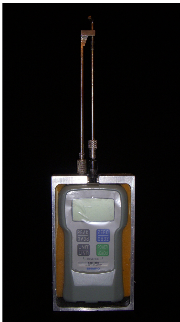
Figure 1 The Digital Force Gauge and its components.
