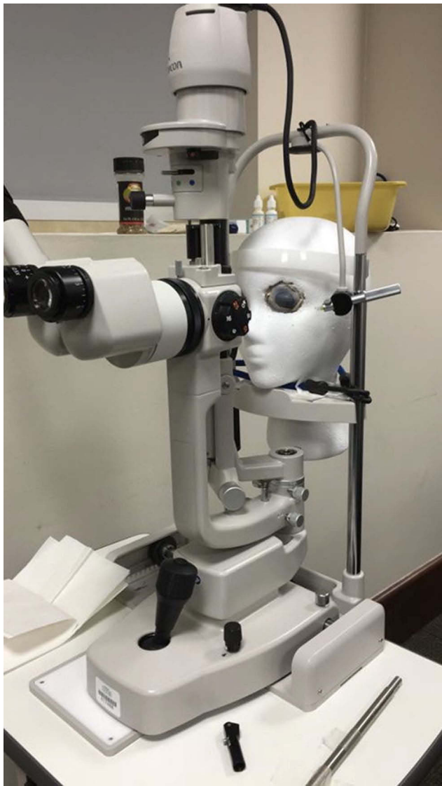
Figure 2 The example of the harvested cow eye and styrofoam head models mounted in the Slit-Lamp.
