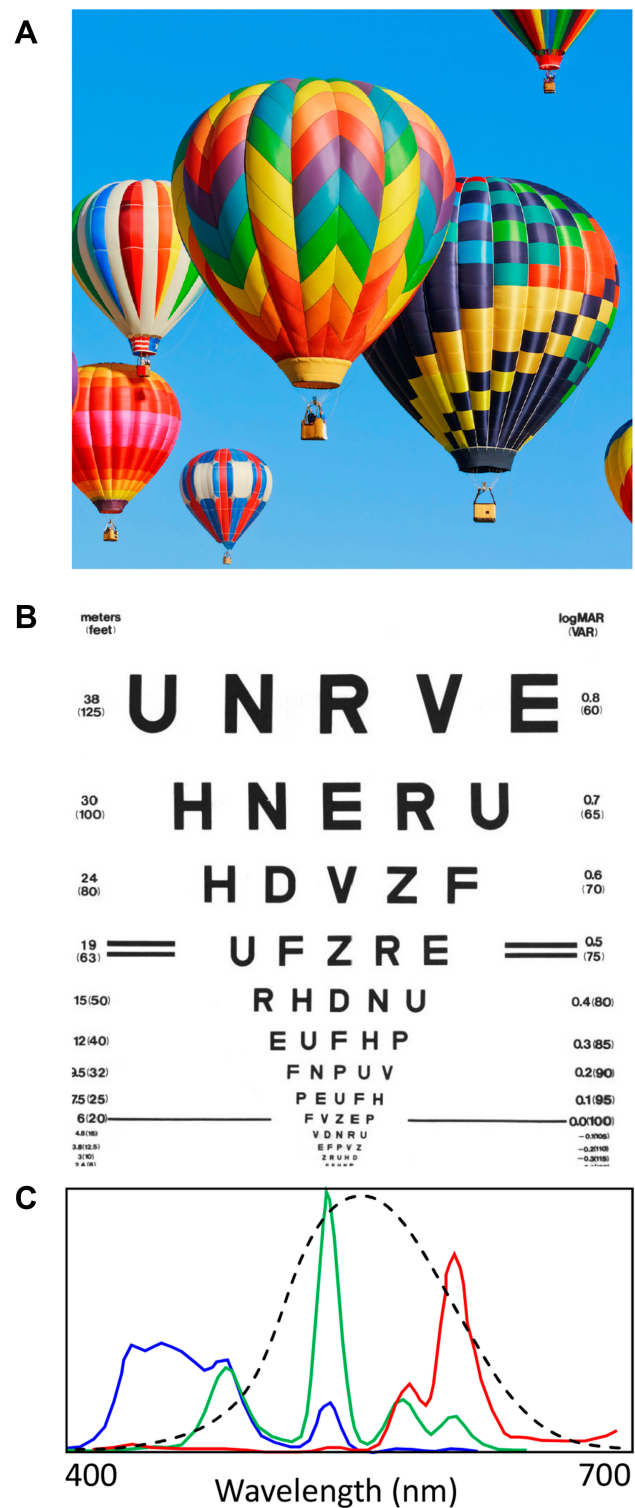
Figure 1 Two source images used for optical modeling. (A) A 3.4 x 3.4 degree colored image represented by three color planes (RGB). (B) A white light image of a 5 x 5 degree logMAR chart that can be represented as three separate RGB spectra (colored lines in C) or a single flat white spectrum. The human spectral sensitivity curve is plotted in (C) (black dashed line).
