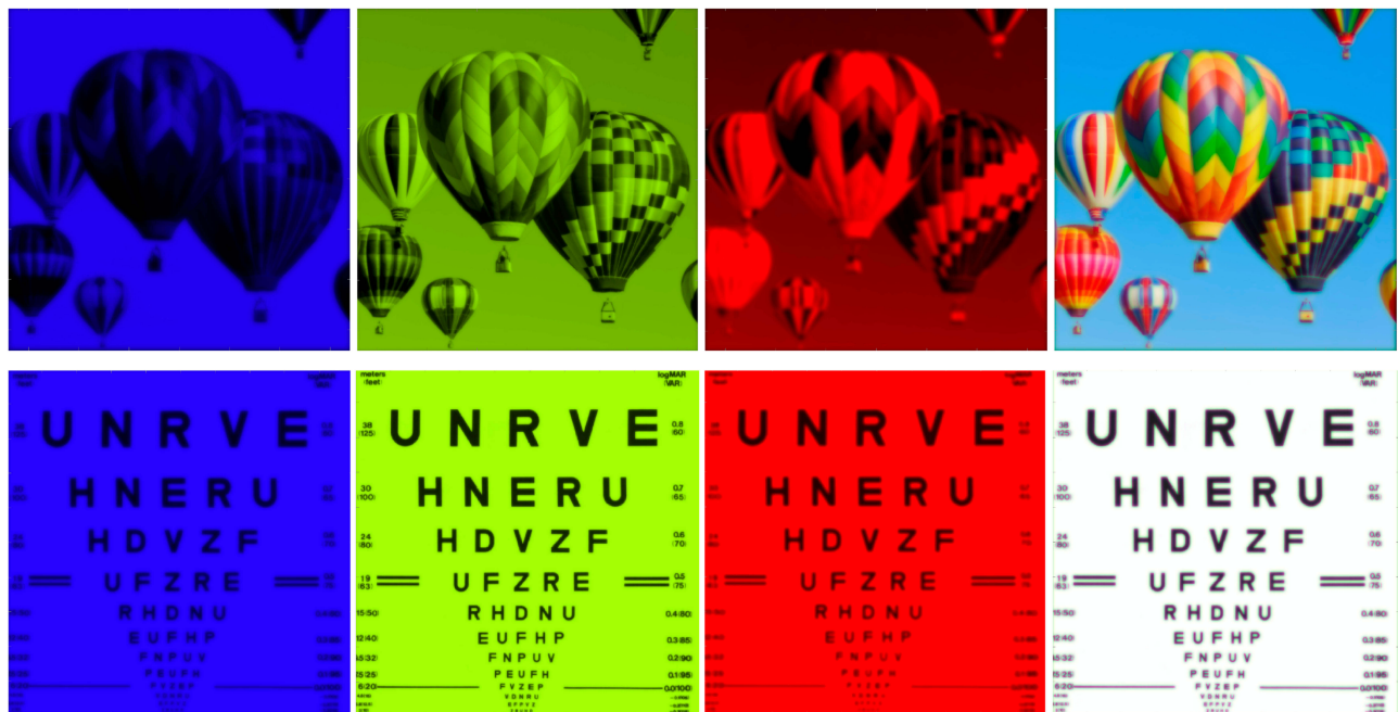
Figure 3 Examples of simulated retinal images with CRT spectra after V_\lambda weighting has been applied to each monochromatic PSF. Top row a highly colored object subtending 3.4 degrees, and bottom row a white object subtending 5 degrees of visual angle (logMAR 0.00 letters subtend 5 arc minutes). Model includes LCA of a phakic eye model, zero monochromatic aberrations.
