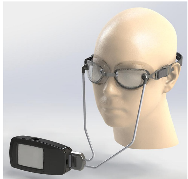
Figure 1 This figure demonstrates the multi-pressure dial, which includes the goggles connected to a pressure-modulating pump. This device was worn nightly by subjects for 7 consecutive nights during the study.
