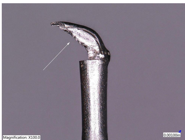
Figure 2 TrabEx blade, featuring two serrated blades (arrow) without a non-cutting ramp.
