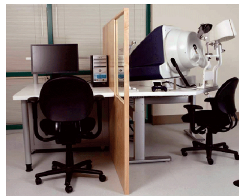
Figure 6 The IRay system set up within the clinical environment with the operator controls separated by the lead-lined glass screen.
