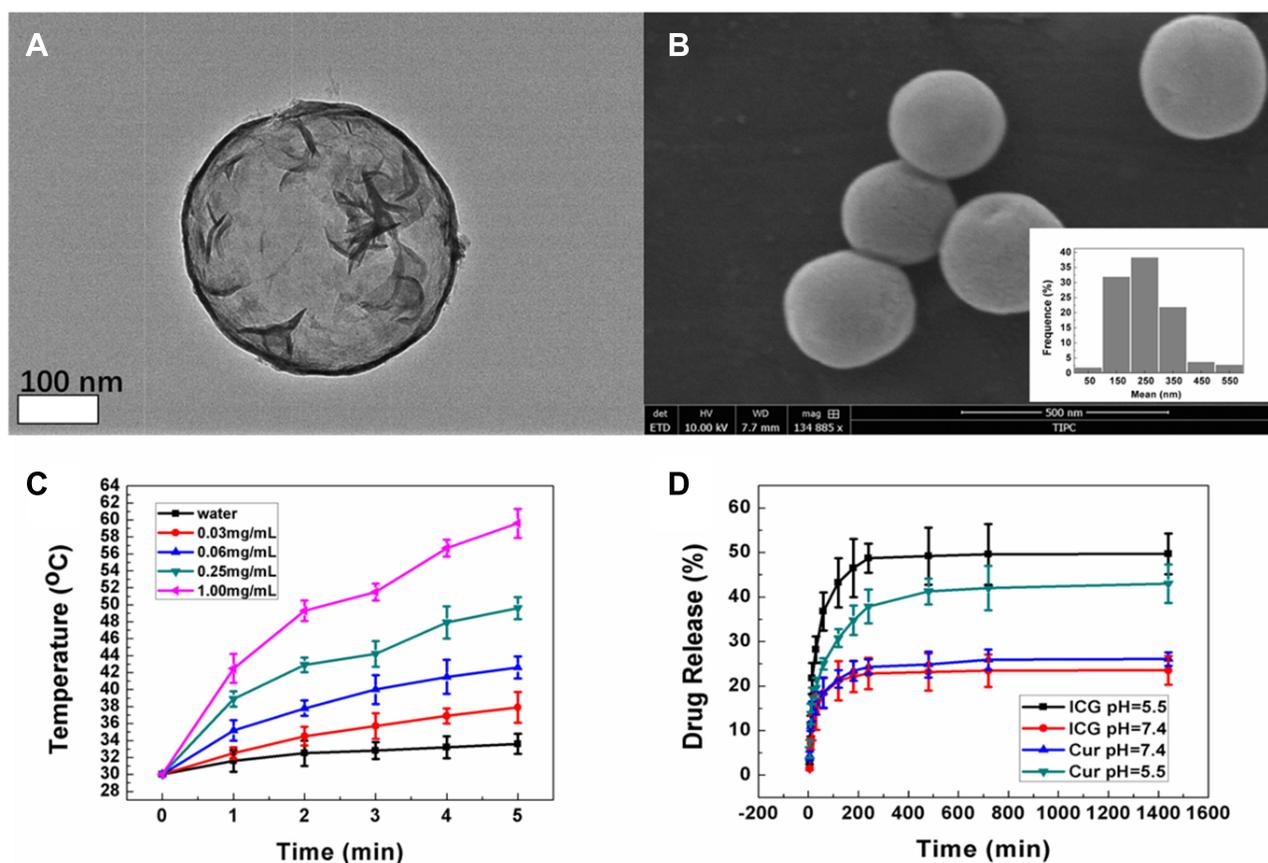
**Figure 1** (A) The TEM image of LMHSs. (B) The SEM image and the average size of LMHSs. (C) In vitro temperature elevation curves of the ICG&Cur@MoS<sub>2</sub> NPs made at different concentrations under irradiation of an 808 nm NIR laser. (D) Drug release of ICG&Cur@MoS<sub>2</sub> NPs under different pH values.
