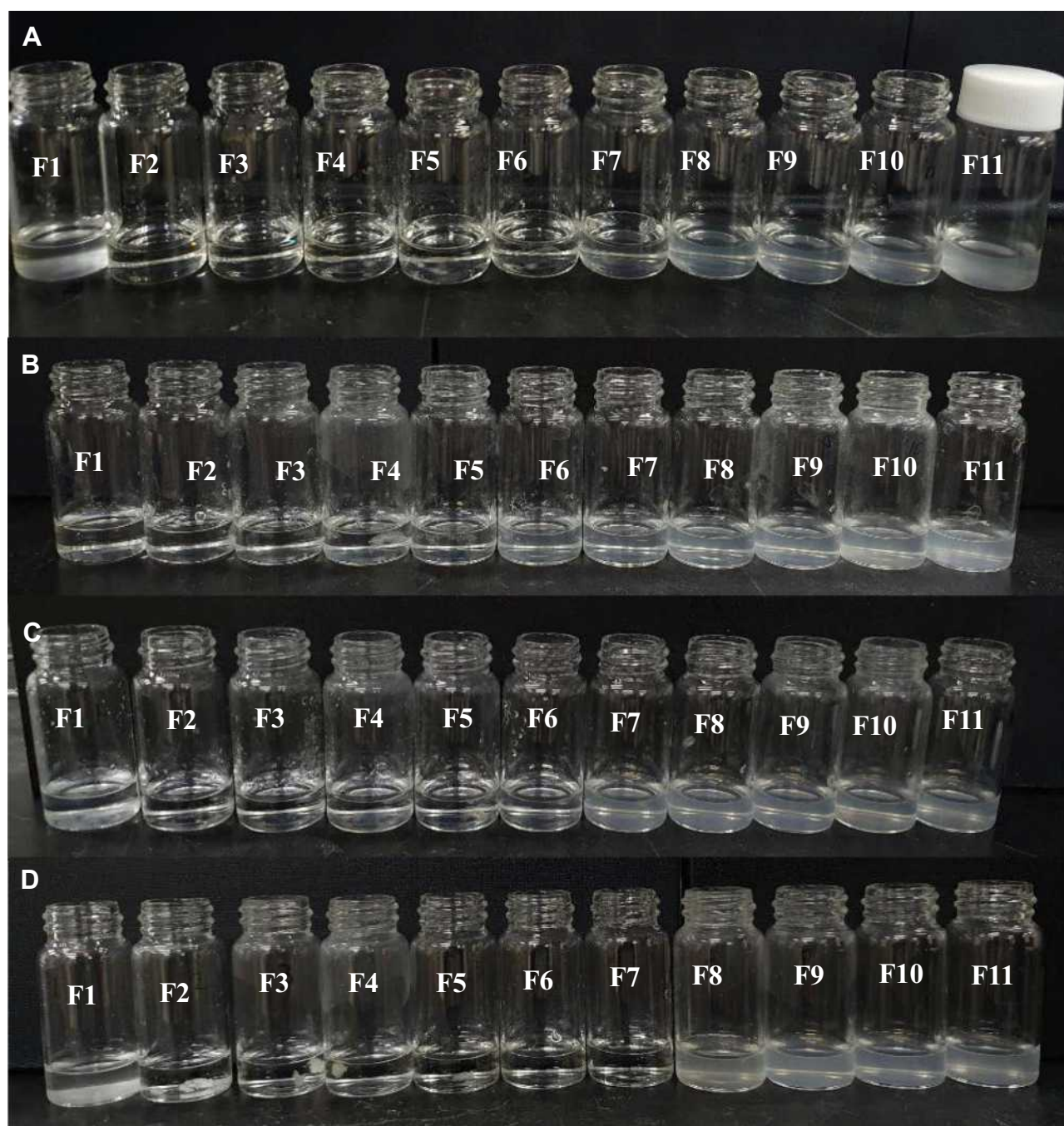
Figure 4 Dispersion images of AOC in various ratios of water with (A) NMP, (B) DMSO, (C) ethanol, and (D) THF solvent.
