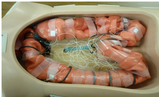
Figure 1 The top view of the Active Colonoscopy Training Model. 15 The base is the conventional colonoscopy training model with an artificial ex vivo colon, and 10 low profile load cells, 24 light sensors, and pressure transducers are integrated with the drivers and the data acquisition system.
