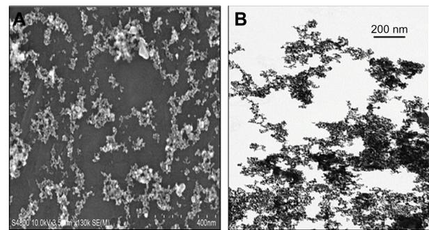
**Figure 1** Characterization of the cerium oxide nanoparticles by (A) field emission scanning electron microscopy and (B) transmission electron microscopy (scale bar = 200 nm) of a dilute cerium oxide suspension.
