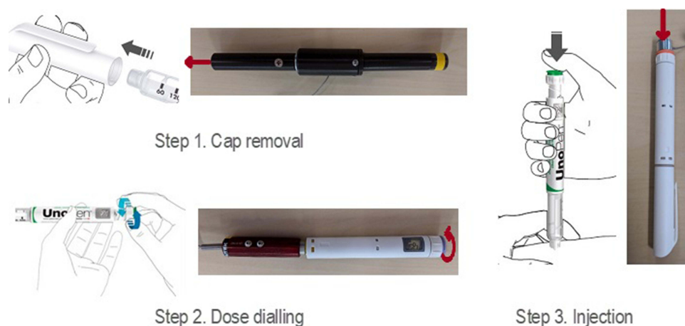
Figure 1 Illustration of handling steps and non-functional dummy devices with force and torque sensors used in the study.
