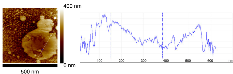
Figure S2 AFM analysis of the height of a liposome/PC complex.
