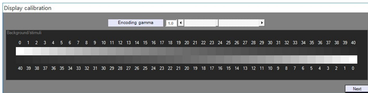
Figure 3 Display – gamma calibration using a gray scale step-wedge.
