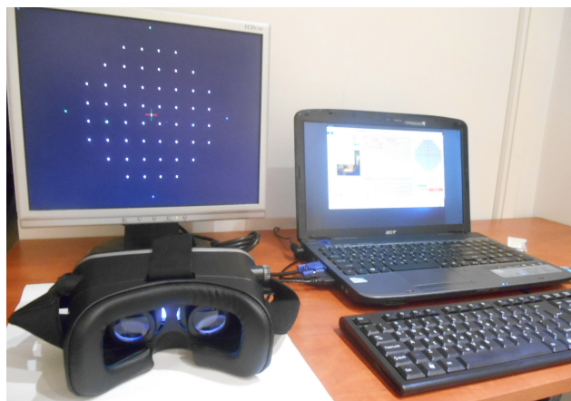
Figure 2 Monitor or virtual reality glasses can be used for visual field testing.
