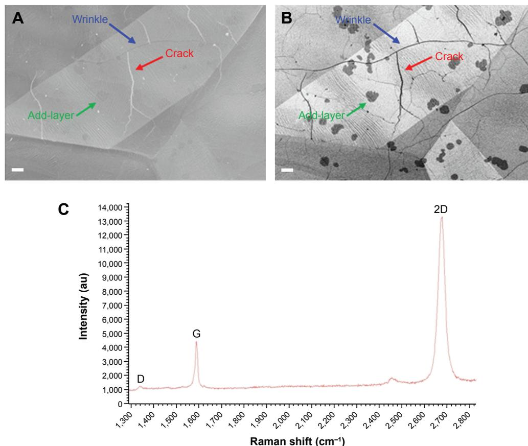
**Figure 3** SEM images recorded using (A) in-lens and (B) ESB detectors with the graphene features marked: the scale bars are 2  $\mu\text{m}$ . Reprinted from Pasternak I. Synthesis and properties of graphene obtained on metallic and germanium substrates by CVD method [unpublished PhD thesis]; 2016; Copyright © 2016 Pasternak. (C) Raman spectra of the graphene.
