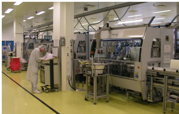
Figure 7 Part of the production line for the automatic assembly of the Respimat® Soft Mist™ Inhaler.
