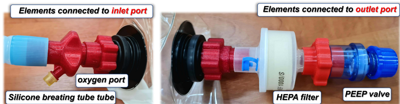
Figure 16 The main view of the inlet and outlet fitting elements mounted in the helmet ports.
