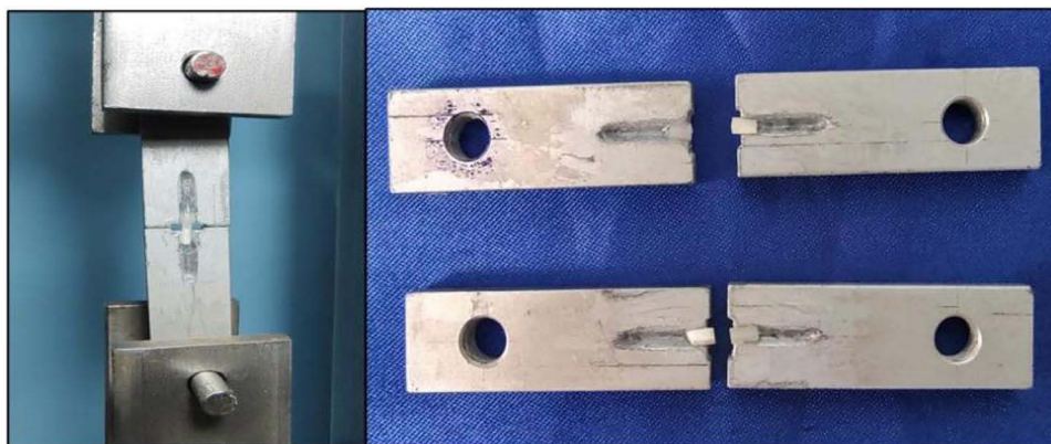
Figure 3 Microtensile bond strength testing.
