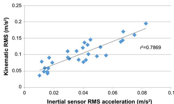
**Figure 2** Correlation between the inertial sensor and rigid-body motion.
