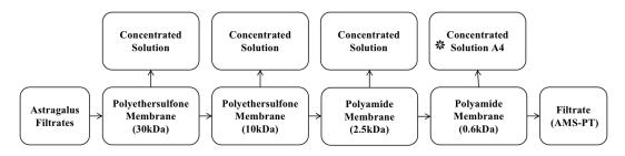
Figure I Flow chart of Astragalus membrane separation process.
