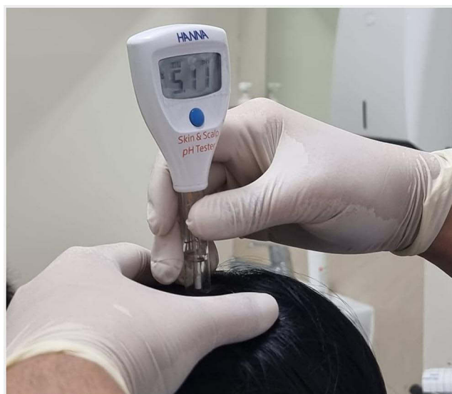
Figure 3 Scalp pH values were measured using a Skin & Scalp pH Tester Hanna Instruments® HI981037.
