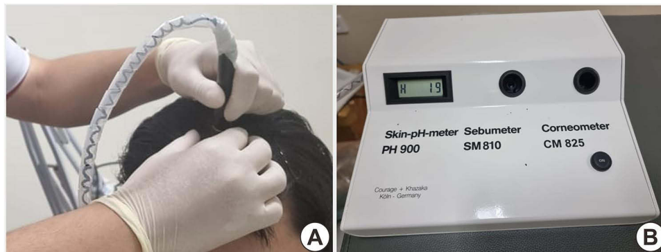
Figure 2 Scalp hydration values were measured using a Corneometer ® CM825. (a) The probe was placed vertically. (b) The monitor showed the scalp hydration values.
