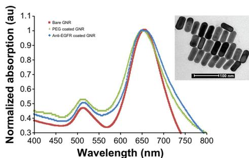
**Figure 2** Ultra-violet visible absorption spectra (normalized) of bare GNRs (25 nm  $\times$  65 nm), PEG-coated and anti-EGFR-coated GNRs, and transmission electron microscopy image of the bare GNRs (inset).
