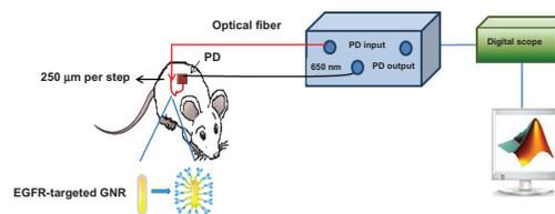
**Figure 1** A schematic description of the experimental setup for the reflected light intensity measurements. Laser diode (650 nm) and an optical fiber (arrow) were used to irradiate the sample on a single point. The photodiode was in close contact with the sample surface. The micrometer plate moved in 20 incremental steps of 250  $\mu\text{m}$ , enabling continuous measurements of the spatial reflectance from the sample, from 1 mm up to 6 mm from the laser diode position.
