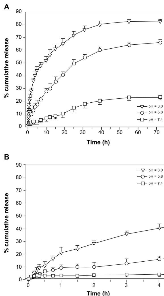
**Figure 8** Release profiles of etoposide from ESCNs under simulated physiological conditions. **(A)** Release profiles of etoposide from ESCNs under simulated physiological conditions (pH 3.0, pH 5.8, and pH 7.4 at 37°C); **(B)** release profiles in the initial 4 hours.
