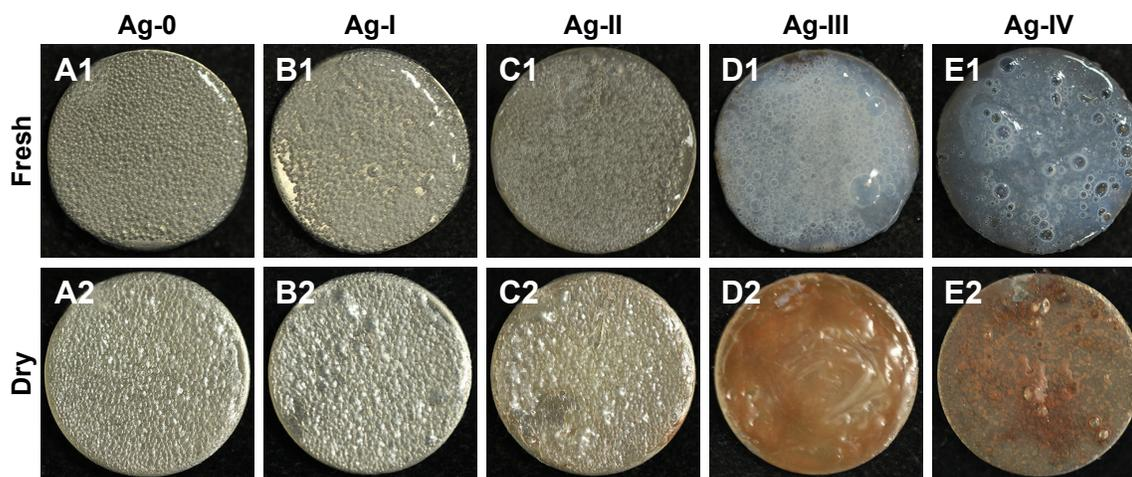
**Figure 1** The optical photographs of fresh (A1–E1) and dry (A2–E2) CS/G and Ag-containing nanocomposite coatings.
