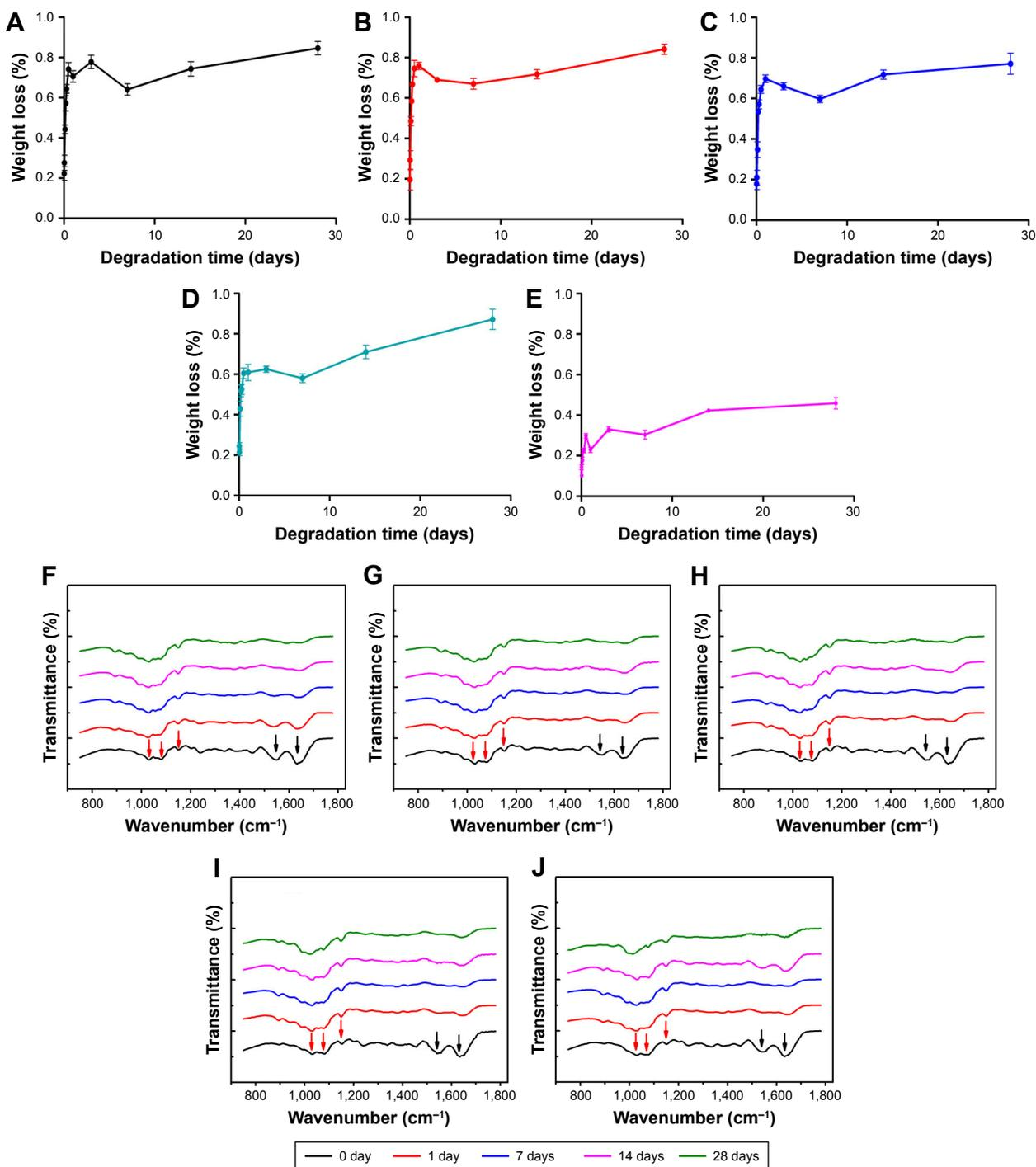
**Figure 6 (A–E)** Degradation rate of CS/G and Ag-containing nanocomposite coatings in PBS under sterile condition ( $n=4$ ) and **(F–J)** ATR-FTIR spectra of CS/G and Ag-containing nanocomposite coatings after degradation in PBS at specific times: 0, 1, 7, 14, and 28 days (red arrows: peaks corresponding to chitosan; black arrows: peaks corresponding to gelatin): **(A and F)** Ag-0, **(B and G)** Ag-I, **(C and H)** Ag-II, **(D and I)** Ag-III, and **(E and J)** Ag-IV.
