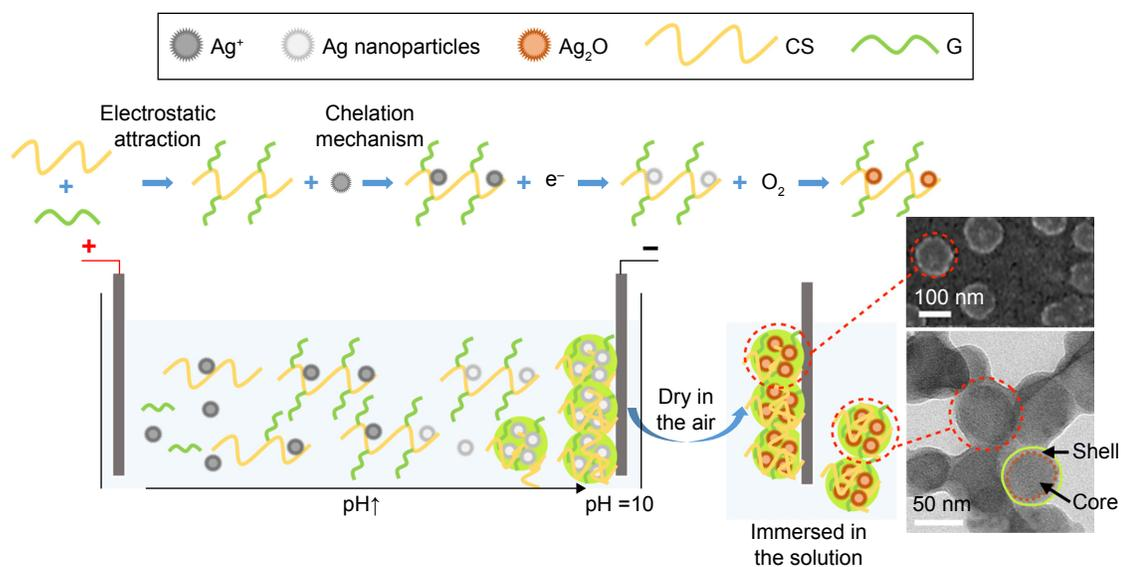
**Scheme 1** Fabrication process of Ag-containing nanocomposite coating via EPD. Ag-containing nanoparticles were formed as shown in the SEM result. TEM results revealed a core–shell-like structure of the released nanoparticles.
