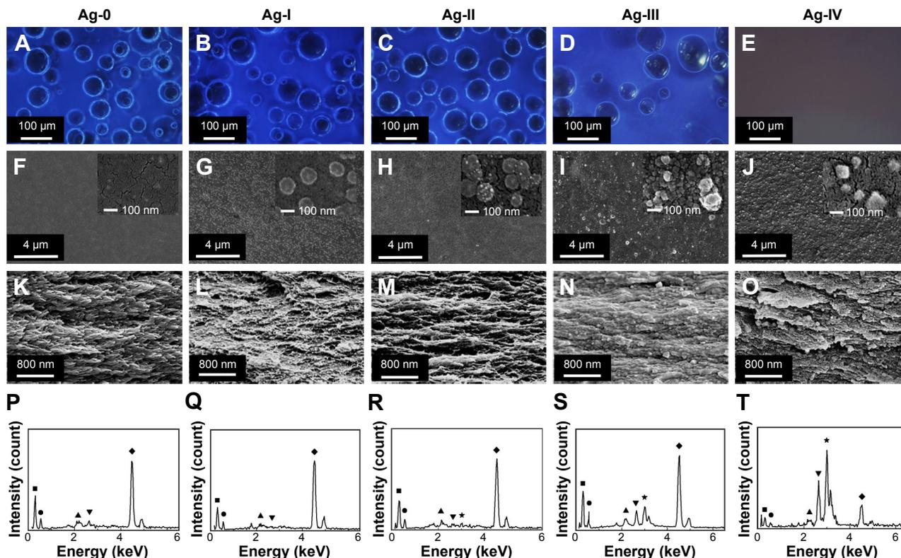
**Figure 2 (A–E)** The fluorescence images, **(F–J)** SEM images of surface with low and high magnification, **(K–O)** SEM images of cross-section, and **(P–T)** EDS spectra of CS/G and Ag-containing nanocomposite coatings (square: C, circle: O, triangle: Au, inverted triangle: Cl, star: Ag, diamond: Ti).
