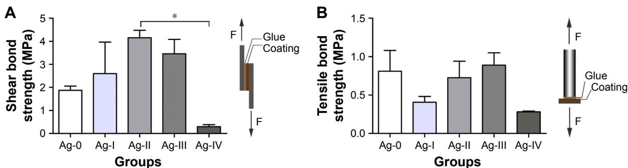
**Figure 5** Bar graph of the (A) shear and (B) tensile bond strength of CS/G and Ag-containing nanocomposite coatings on titanium surface (n=3; \*P<0.05). **Abbreviations:** CS/G, chitosan/gelatin; F, force.
