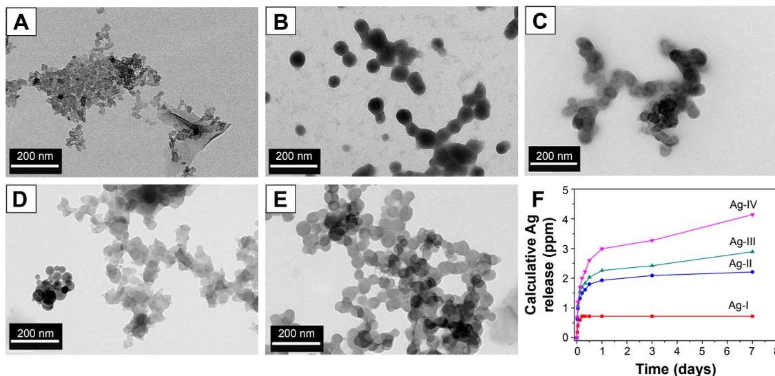
**Figure 4** TEM images of the released nanoparticles and calculative release profiles of Ag ions from CS/G and Ag-containing nanocomposite coatings in PBS: (A) Ag-0, (B) Ag-I, (C) Ag-II, (D) Ag-III, (E) Ag-IV, and (F) release profile. **Abbreviations:** TEM, transmission electron microscopy; CS/G, chitosan/gelatin; PBS, phosphate-buffered saline.
