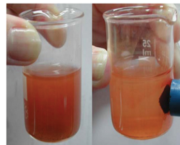
Figure 3 Magnetite-hexane suspension attached to a magnet.
