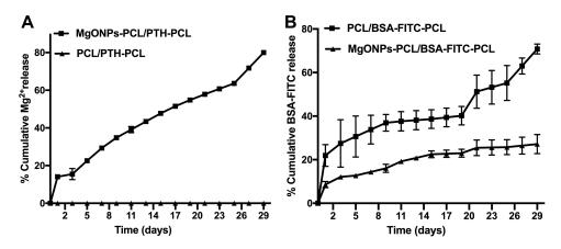
Figure 4 The release profiles of (A) Mg<sup>2+</sup> and (B) BSA-FITC from different membranes for 29 days.
