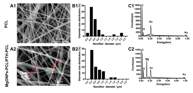
Figure 2 SEM image (A1, A2), fiber diameter distribution (B1, B2) and EDX spectra (C1, C2) of PCL and MgONPs-PCL/PTH-PCL membranes.
