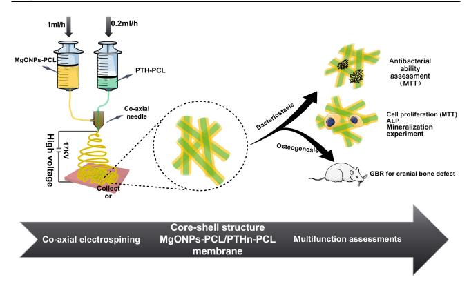
Figure 1 Scheme of preparation and functional assessments of MgONPs-PCL/PTHn-PCL coaxially-electrospun barrier membrane.
