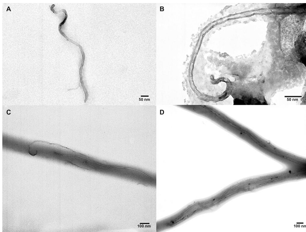
Figure 3 Transmission electron microscopic images. Electrospun (A) SWNT, (B) MWNT, (C) SWNT-10PU, and (D) MWNT-10PU. Abbreviations: MWNT, multiwalled nanotubes; SWNT, single-walled nanotubes; 10PU, 10% w/v polyurethane.
