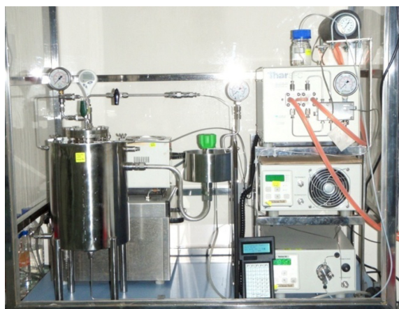
Figure 1 Equipment set-up used in this study for supercritical antisolvent system.
