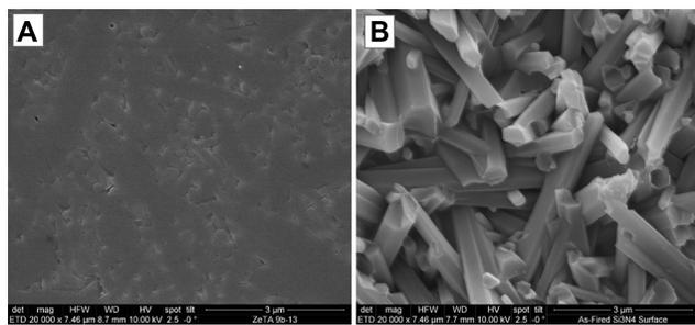
**Figure 2** Scanning electron microscopy surface microstructure of polished and as-fired Si<sub>3</sub>N<sub>4</sub>: (A) polished surface 20,000 $\times$ ; (B) as-fired surface 20,000 $\times$ .
