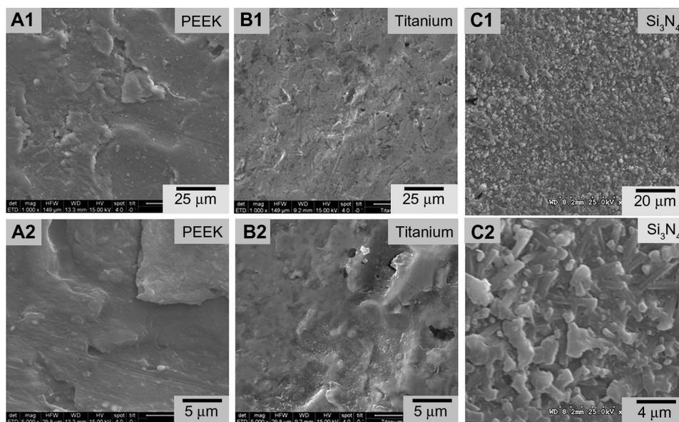
**Figure 1** Scanning electron microscopy surface microstructures of PEEK Optima®, Ti, and Si<sub>3</sub>N<sub>4</sub>; (A1) PEEK 1000×; (A2) PEEK 5000×; (B1) Ti 1000×; (B2) Ti 5000×; (C1) Si<sub>3</sub>N<sub>4</sub> 1000×; (C2) Si<sub>3</sub>N<sub>4</sub> 5000×.
