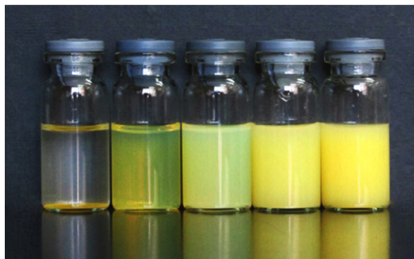
Figure 1 Suspensions of bulk drugs and naked coenzyme Q_{10} nanocrystals of different sizes after storage for 2 days at room temperature.
