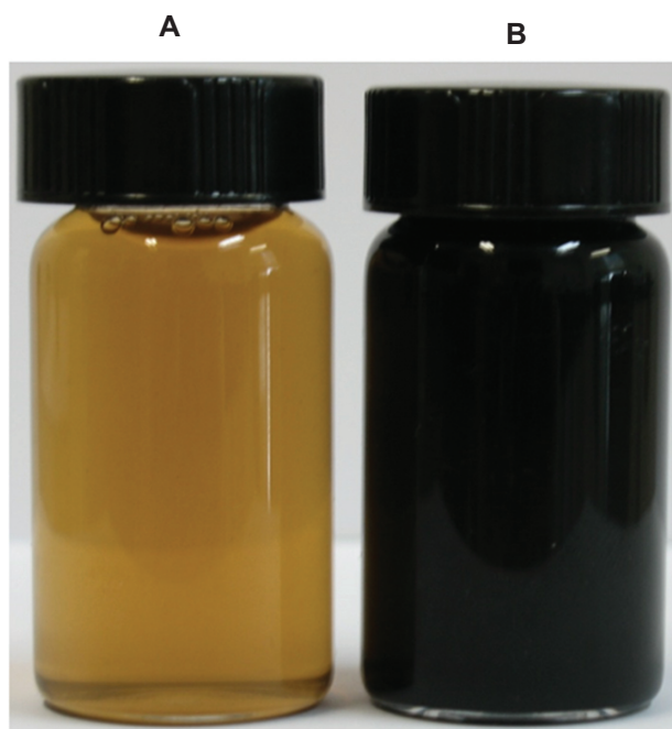
Figure 1 Digital photographs of aqueous dispersions of GO before and after reduction with TEA.
